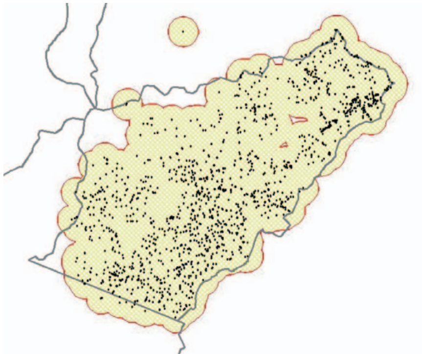
Figure 4 – Distance map defined on the basis of 300 meter coverage radius around each PUT.
